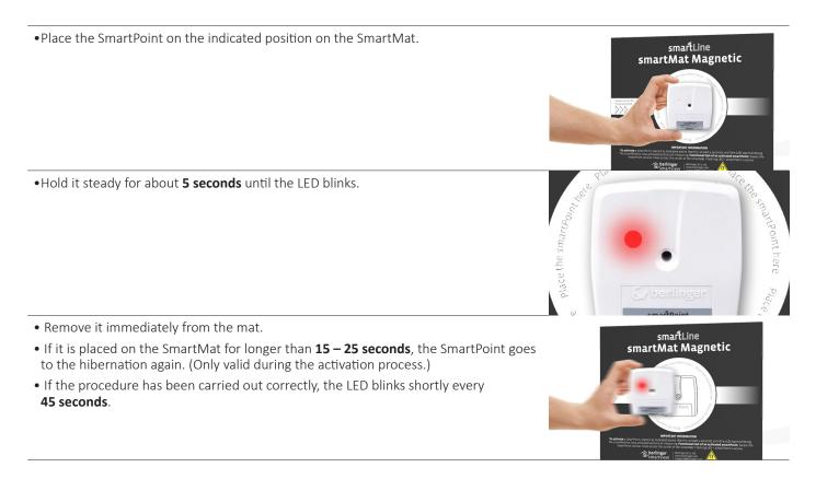
Information: Sometimes the activation of the SmartPoint is not successful e.g. due to movement of the SmartPoint. Retry the activation procedure after 15 minutes.
