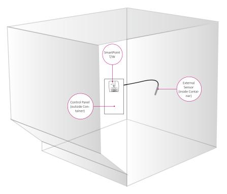
Install the SmartPoint T/1W with external temperature sensor as depicted above.
