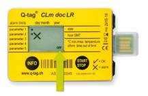
**2.** If the **device is OK, press the START/STOP** button for 3 seconds to activate the device. The OK symbol will be shown and a small black point starts flashing.
