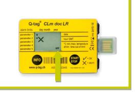
If the **device** is **OK**, **press the START/STOP** button for 3 seconds to activate the device. The OK symbol will be shown and a small black point starts flashing.
