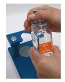
2. Place the metal break cap onto the security cap.
